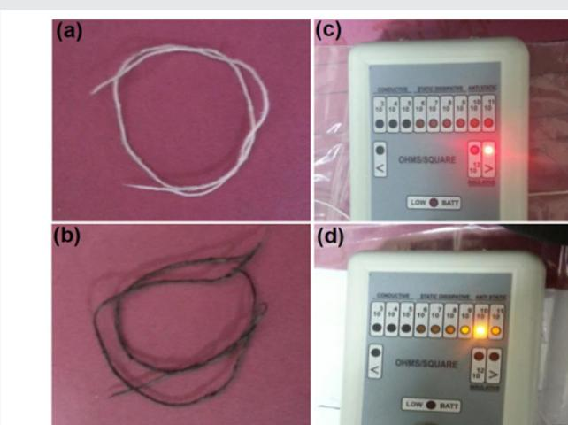
**Figure 4:** Optical image of (a) bare fiber & (b) FCNTs coated fiber; and surface resistivity of (c) bare fiber & (d) FCNTs coated fiber.
