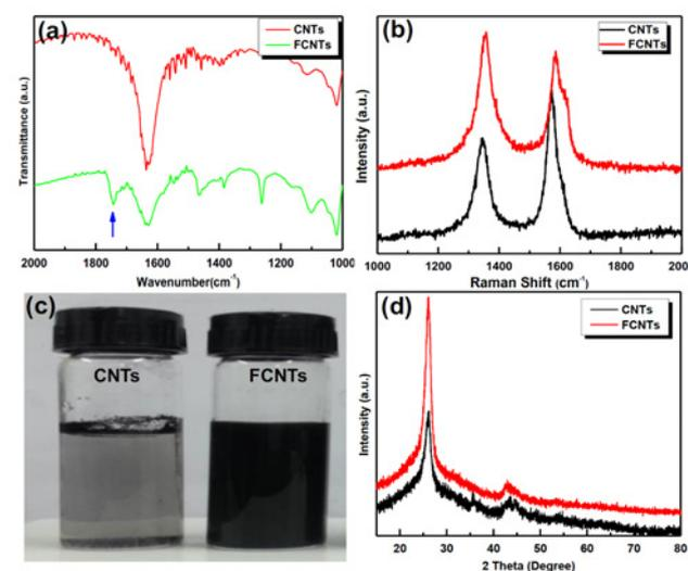
Figure 2: (a) FTIR spectra (b) Raman spectra (c) Dispersion images and (d) XRD Spectra of CNTs and FCNTs.
