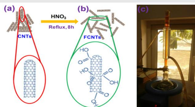
Figure 1: Schematic representation of (a) Pristine CNTs (b) functionalized CNTs (FCNTs); and (c) actual refluxing setup.
