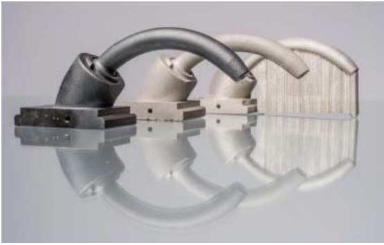
Figure 1: Metal alloy of a lasermelted core for an injection mould of a nasal douche.
