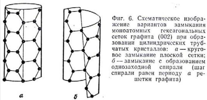
**Figure 2:** Schematic representation of two different arrangements of graphene hexagonal nets (002) rolled into a cylinder, published in [4]: (a) armchair tube, (b) chiral tube (the helix pitch is equal to the corresponding lattice parameter of graphite).
